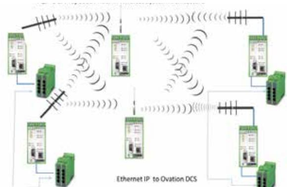
a primary/secondary radio arrangement was made which would allow for communication in the event of individual radio failures. Also included were voltage and current sensors to alert the end user if battery voltage or charging current went below specified criteria.
