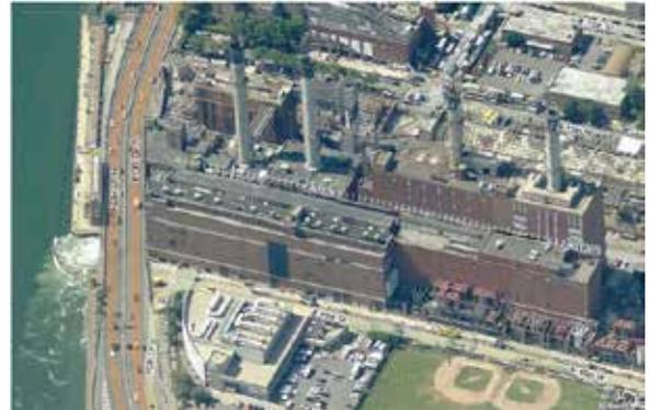
The data from this new system needed to be monitored by the Distributed Control System within the main plant, which was across a highway and about a quarter mile away at a change of elevation of seven stories. Running a new data line via traditional wiring or fiber was cost-and time-prohibitive.
