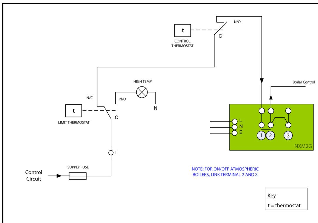
**FIGURE 4. Typical Wiring for single stage forced draft burner**
