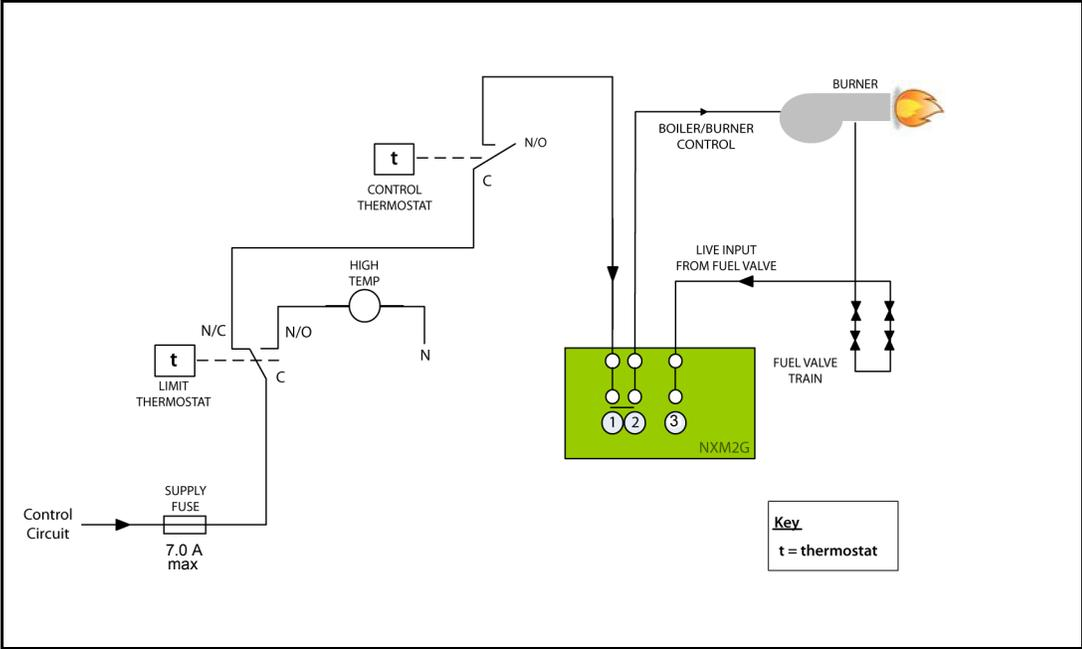
**FIGURE 5. Typical Wiring for 2 stage High/Low force draft boiler**
