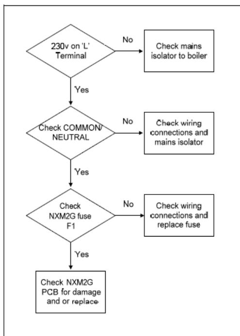
**FIGURE 7.2** NXM2G Power supply correct (red LED on), however boiler will not fire during “First Firing”
